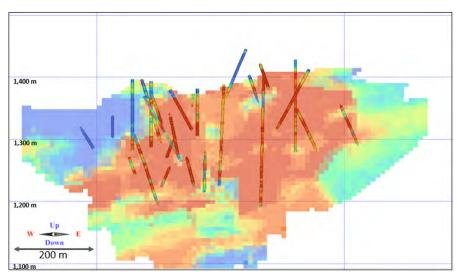
Figure 14.17 Mountain View Project, North-South Block Model Cross Section Visual Checks (Looking North)
