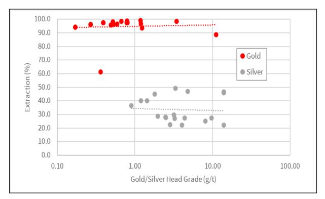
Figure 13.11  $$P_{\$0}$$  75  $\mu m$  Oxide Variability Bottle Roll Tests - Au and Ag Extraction versus Head Grade
