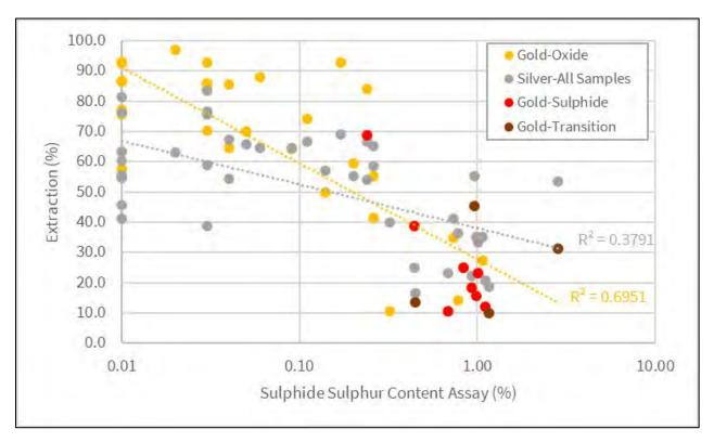
Figure 13.3 P<sub>80</sub> 75 μm Variability Bottle Roll Tests - Au and Ag Recovery versus Sulphide Sulphur Content
