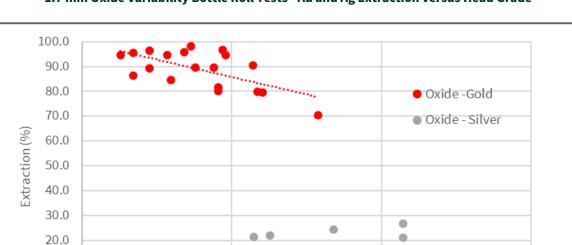
Figure 13.9 -1.7 mm Oxide Variability Bottle Roll Tests - Au and Ag Extraction versus Head Grade
