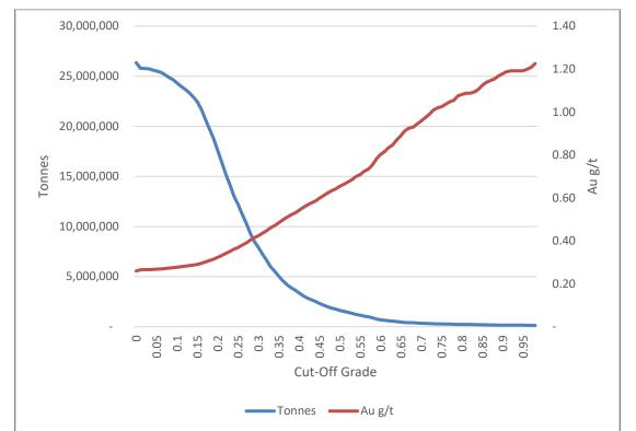
Wildcat Project, Grade Tonnage Curves for the Inferred Mineral Resources at Different Cut-Off Grades
