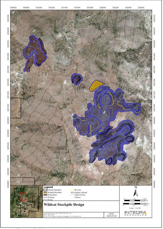
Figure 16.13 Wildcat Project, Mineralized Material Stockpile Design
