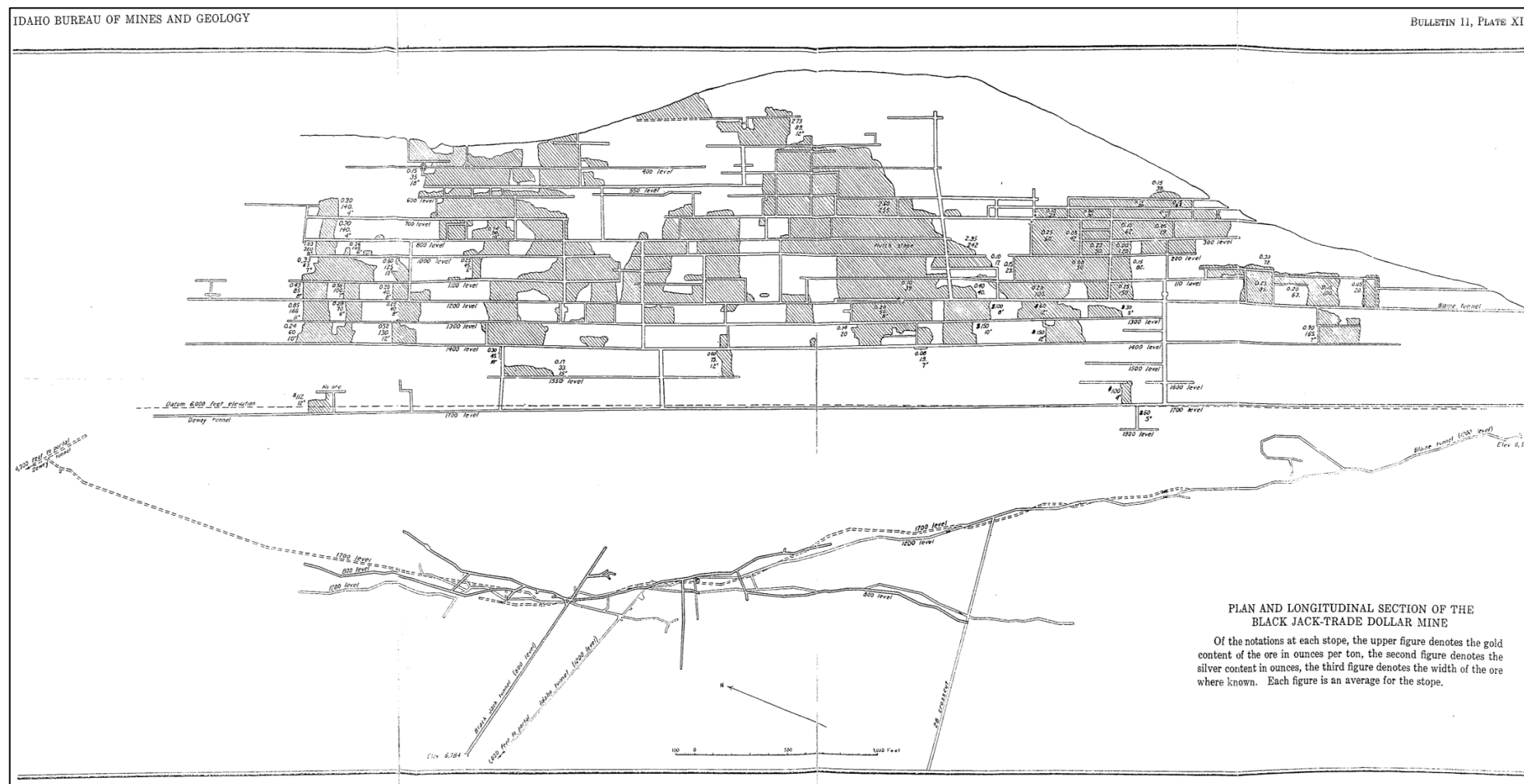
Figure 7-10 Longitudinal Section of the Black Jack – Trade Dollar Mine (from Piper and Laney, 1926)
