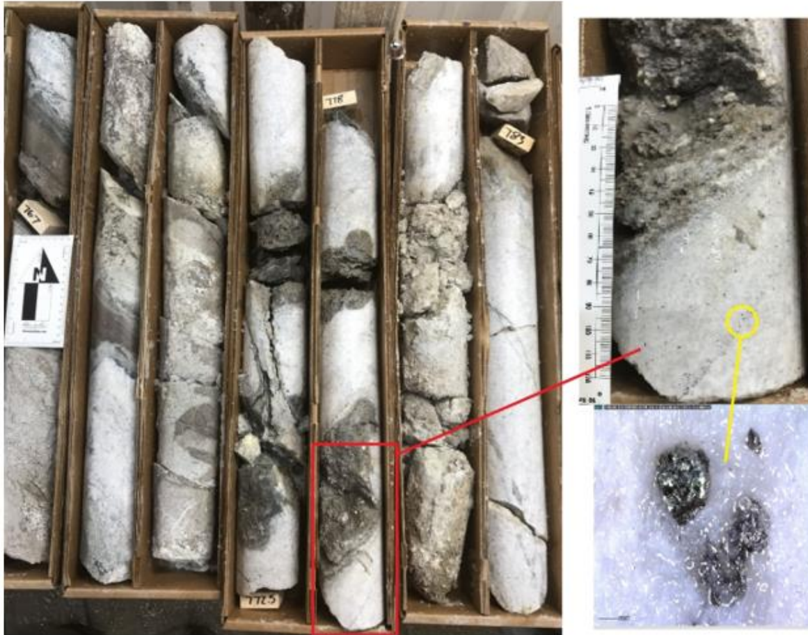
LDE-21-001: Intersect: 767 ft to 783 ft (233.8 m to 238.7 m) - Mineralized quartz-calcite-sulfide vein exhibiting dissolution textures within the quartz. Mineral is a probable form of silver-sulfide.
